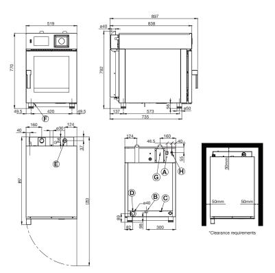
\*Heat Source: 500mm clearance from an external heat source is required in order to protect the oven control components. For clearances under 500mm, it is mandatory for Stoddart heat shields to be fitted while still maintaining a minimum clearance of 50mm to allow access to the unit. Failure to adhere to minimum clearances may void the oven warranty or add service costs due to lack of access.
