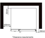
\*Clearance requirements \*Drain line must be vented
