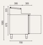
Gross volume: 417 L Exterior dimensions in mm: 1795w x 700d x 1085h Number of adjustable shelves: 3 Gastronorm pan size (top): 8 x GN1/3 Temperature set range: -2°C to +8°C Gross/net weight: 161/130 kg Preparation area material: stainless steel Energy consumption in 24h: 4.35 kWh
