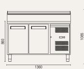
Allow min. 100mm clearance for instalation, all vents must be left clear
