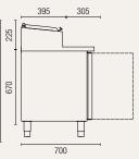
Gross volume: 282 L Exterior dimensions in mm: 1360w x 700d x 1085h Number of adjustable shelves: 2 Gastronorm pan size (top): 7 x GN1/3 Temperature set range: +2°C to +8°C Gross/net weight: 131/104 kg Preparation area material: stainless steel Energy consumption in 24h: 3.4 kWh
