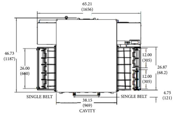
PS638 Top View – Electric & Gas Single Unit
