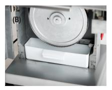
CDE. Lossen the tensioning Knob to relax the band saw then demount the saw (Wearing gloves before ). One hand press down the tensioning knob, one hand upward lift the Driven wheel out and clean
