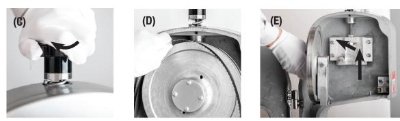
F. Please use low pressure squirt gun to spray the interior minced meat, then reinstallment in order. ▲ Electrical parts(as exterior control knob,switch....) can't be directly sprayed by squirt gun.
